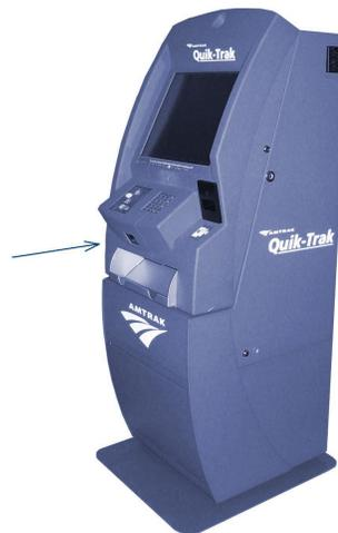
**Simply placing the barcode in front of the red scanner grid as shown will bring up the user's itinerary and allow for the issuing of tickets with one press of the "Print Tickets" button.**
